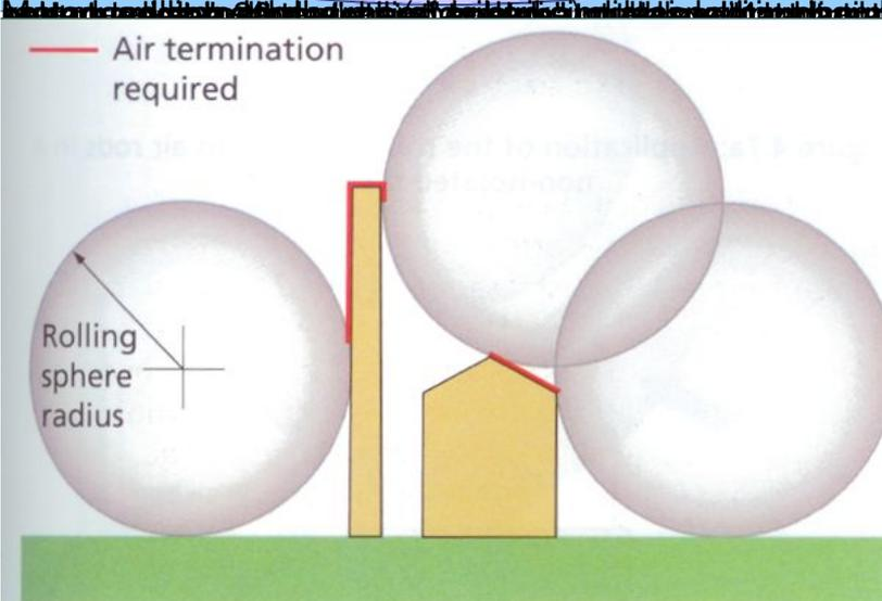
Figure 4.4: Application of the rolling sphere method
